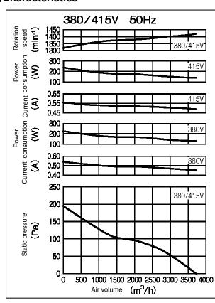
\*The air volume was measured using the orifice chamber method.
